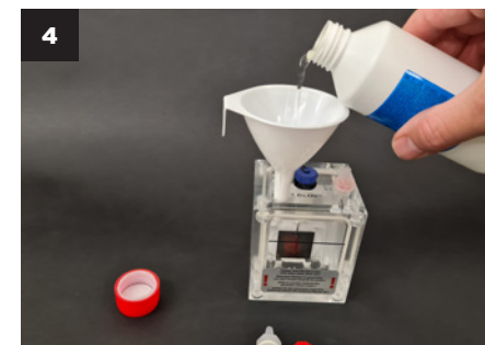
Insert the funnel into the first chamber and pour sodium chlorite up to the line on the generator.
