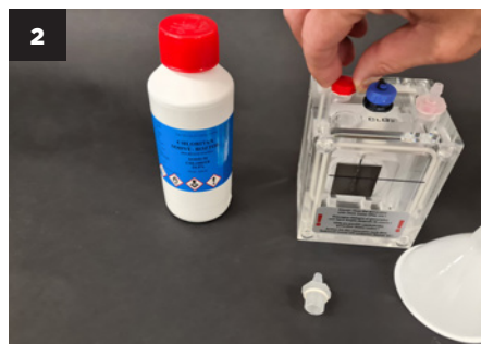
Unscrew the two holes to pour the sodium chlorite into the generator chambers.
